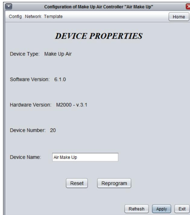
Figure 43 - Device Properties Screen
