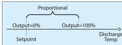
As the discharge air drifts above the setpoint, the Proportional component ramps up the cooling output to compensate.
