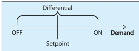
**Figure 30 - Staged Cooling based on Demand**
