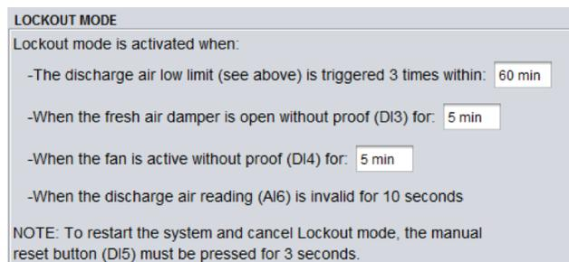
**Figure 41 - Lockout Mode**
