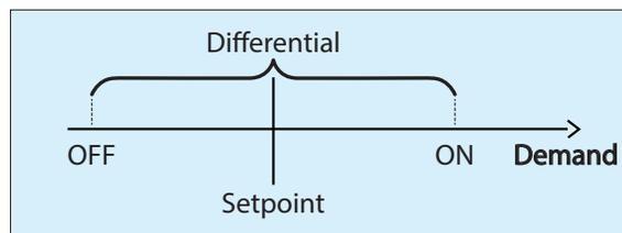
Figure 36 - Valve Differential Control
