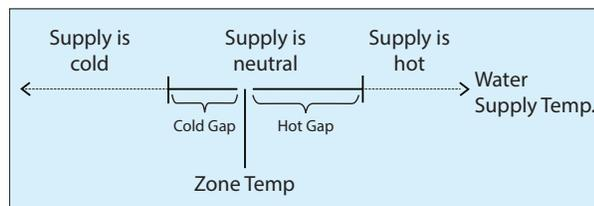
Figure 41 - Thermistor Change Over Ranges
