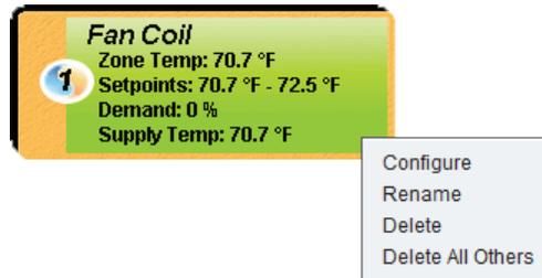
Figure 9 - Icon Right-Click for Fan Coil Unit
