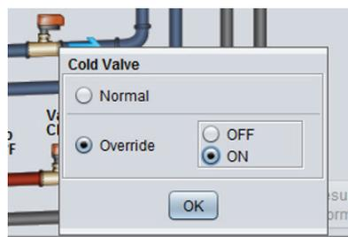
Figure 14 - Manual Override of the Valve
