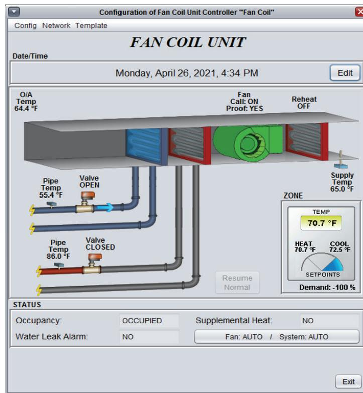
Figure 10 - Fan Coil Unit Controller Home Screen
